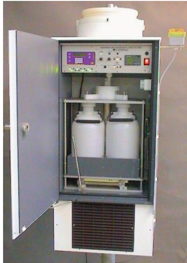
NSA 181/KD - VMM Including data logging system
