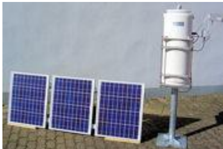
UNS 130/E Low power consumption with solar and/or battery supply
